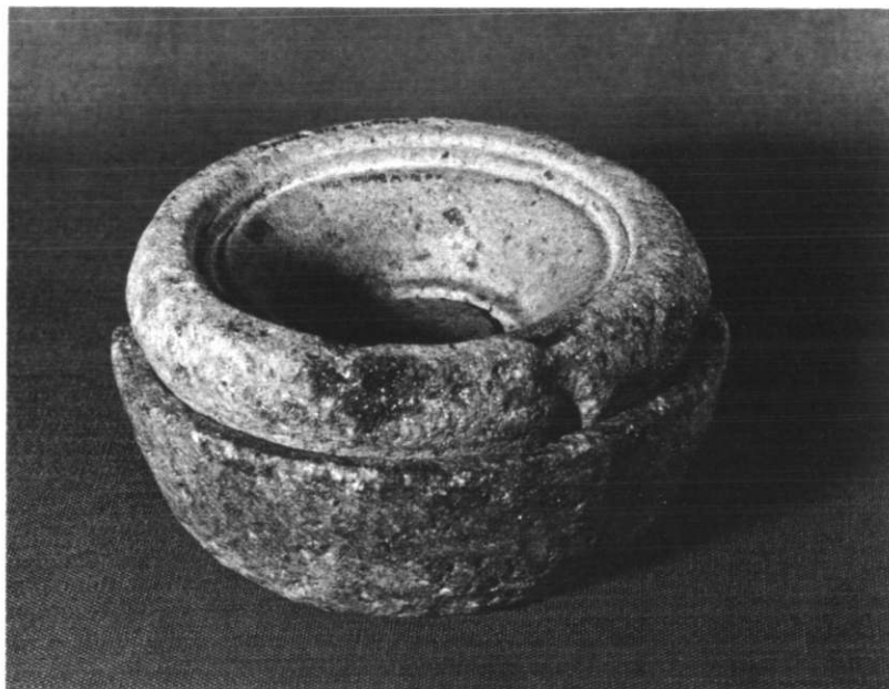
b. The two stones assembled as for casting, with pouring hole in the front
